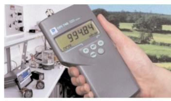
The DPI 740 is a portable battery powered precision barometer, providing outstanding capabilities in a hand held package. The fundamental sensor technology employed within this instrument is the Druck Resonant Pressure Transducer (RPT). This vibrating element sensor not only provides accuracies of ±0.005 inHg but equally important has a calibration stability of better than 100 ppm per year The DPI 740 is widely used in laboratory and remote field applications for precision pressure reference
